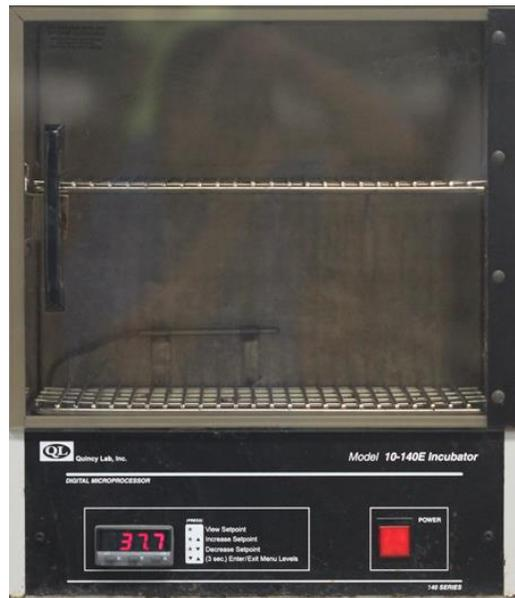
Figura 4. Incubadora model 10-14E incubator.
